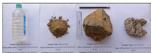
Fig. 9. Samples of materials collected at the site of the structure.
