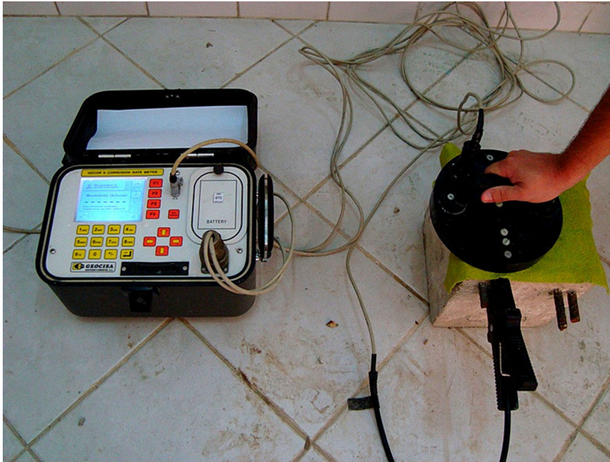
Fig. 3 Measurements of I_c in reinforcement steel in the RC specimens using corrosimeter
