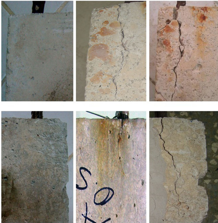
Fig. 8 Visual observation of the RC specimens placed in the coastal outdoor exposure site during three years of study
