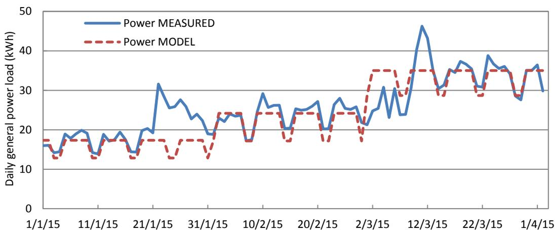
Figure 4-11 TTT equipment power electrical use comparison.
