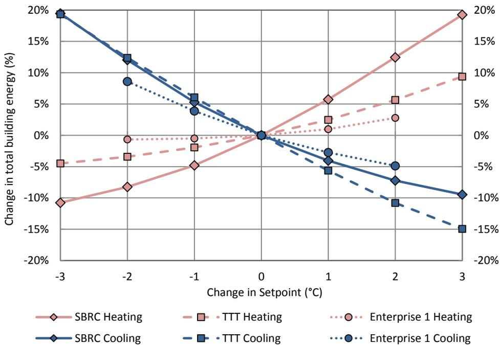
Figure 5-24 HVAC setpoint simulations: change in building energy use.
