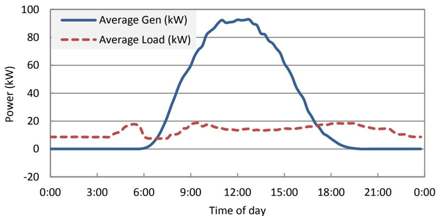
Figure 6-11 SBRC average load and generation profiles: 2015.
