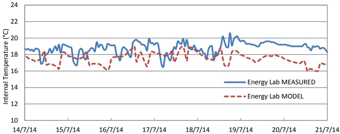
Figure 4-13 SBRC energy lab temperature profile comparison – winter.
