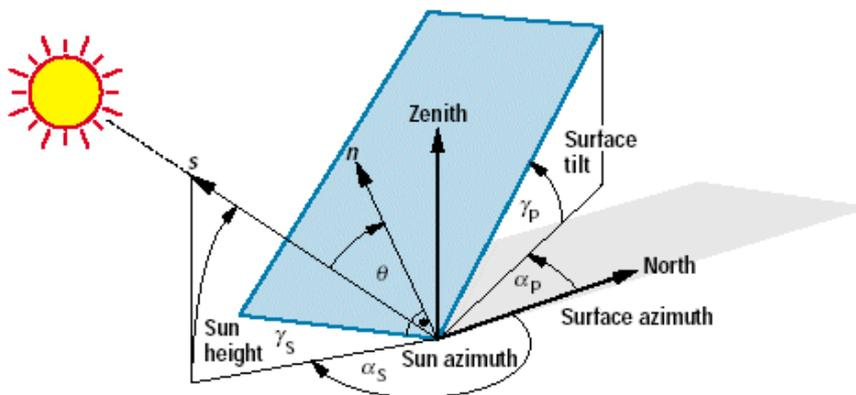
Figure 2-1 Angular relationship between the sun and a tilted flat plane [46].
