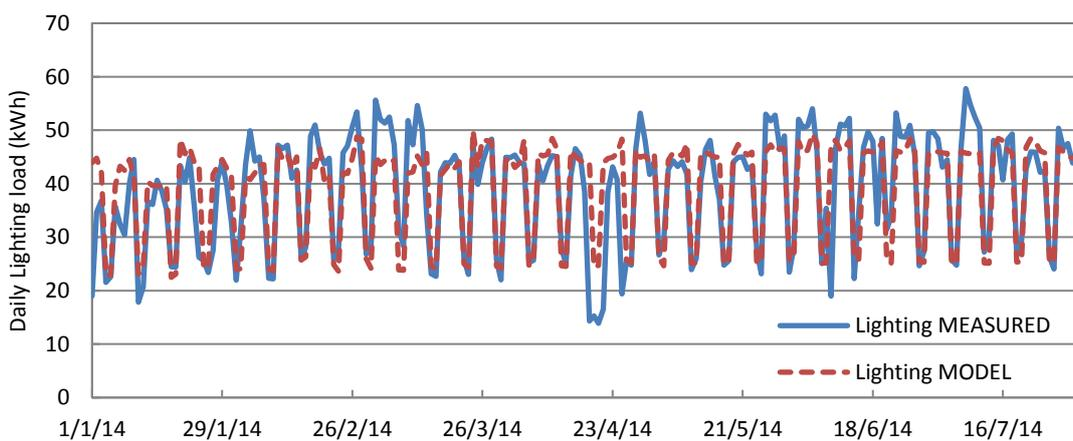
Figure 4-23 SBRC lighting electrical use comparison.
