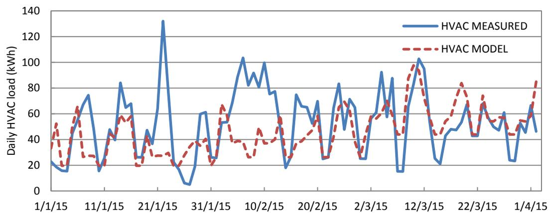
Figure 4-12 TTT HVAC electrical use comparison.
