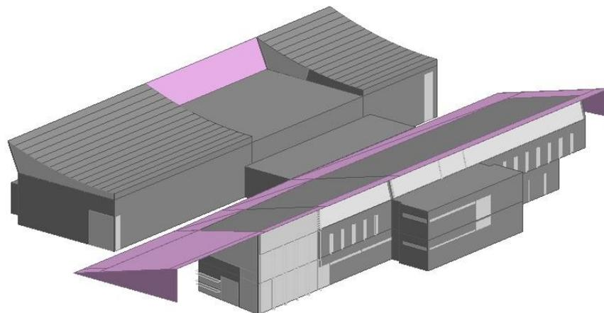
Figure 4-2 SBRC building model physical geometry as modelled in DesignBuilder.
