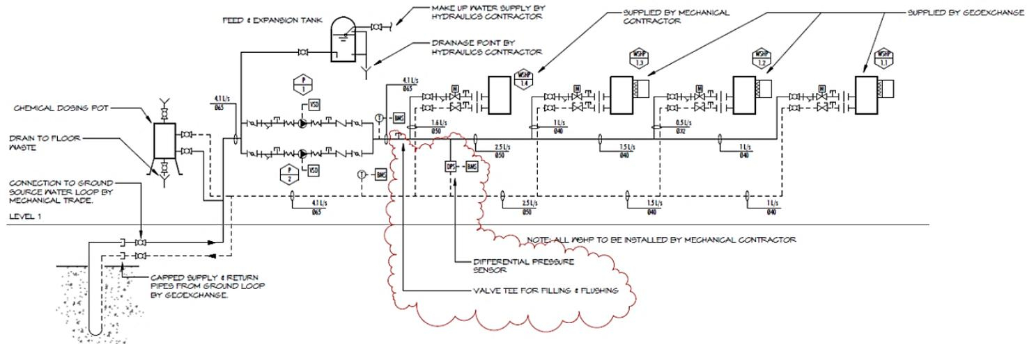
Figure 3-13 TTT building HVAC water services schematic [78].
