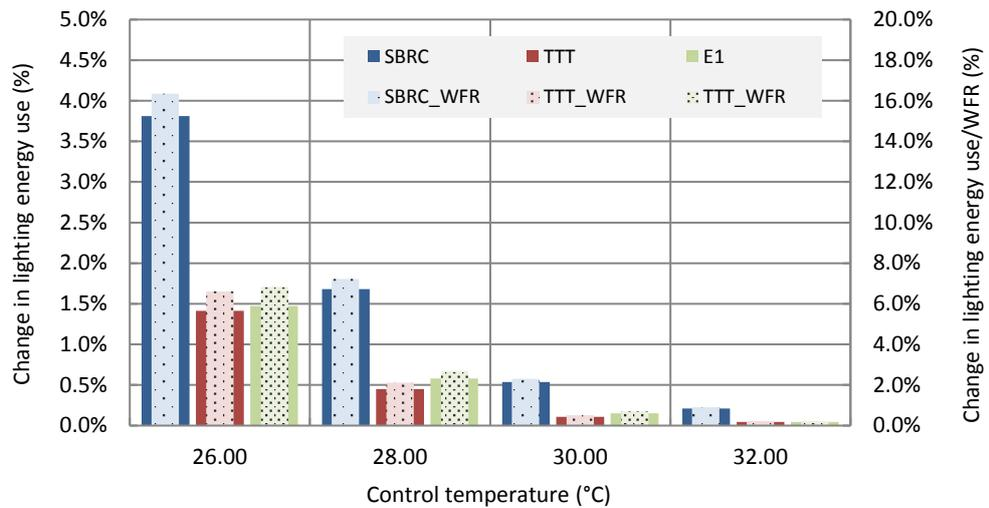
Figure 5-17 Shading simulations: lighting energy use - temperature control.
