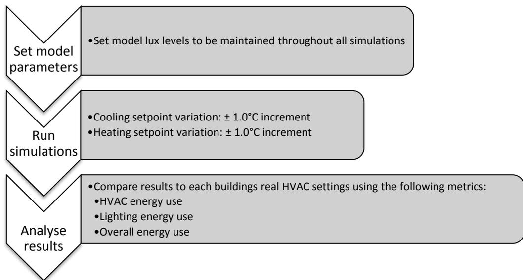
Figure 3-8 HVAC simulation procedure.
