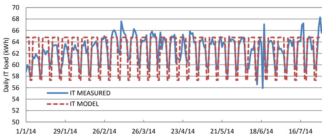
Figure 4-24 SBRC IT electrical use comparison.
