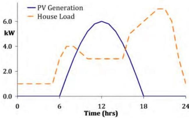
Figure 2-2 Typical load/gen profile for residential building with solar PV - [55]
