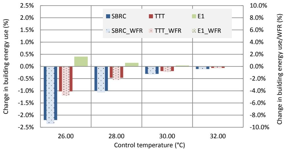
Figure 5-22 Shading simulations: building energy use - temperature control.
