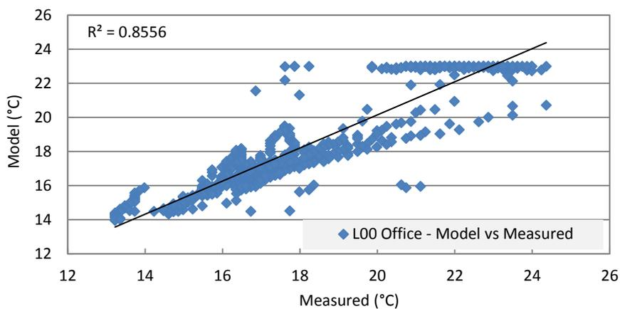
Figure 4-5  $R^2$  for ground floor office temperature comparison.
