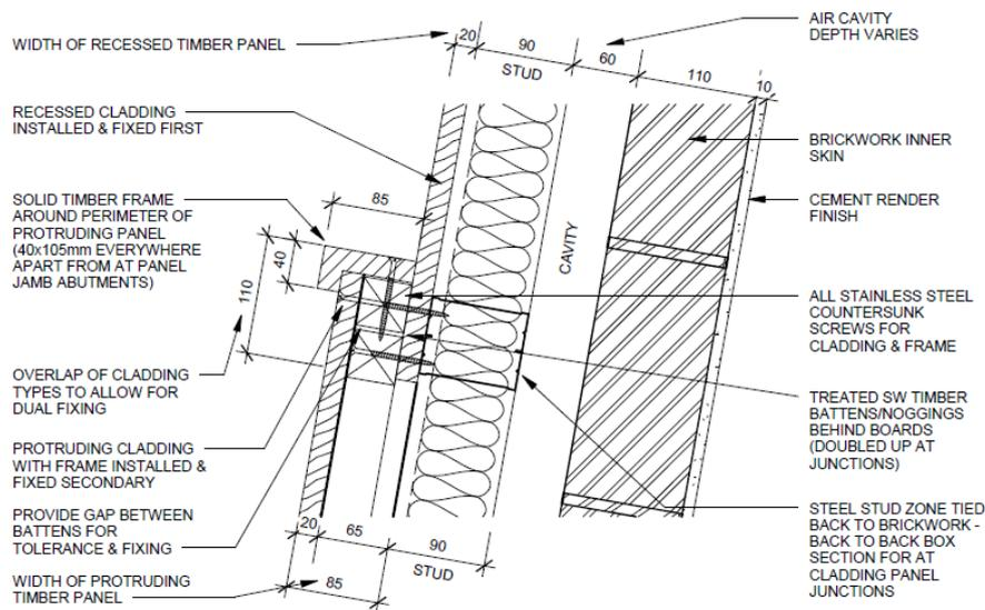
**7** Detail Plan of Timber Cladding Junction
