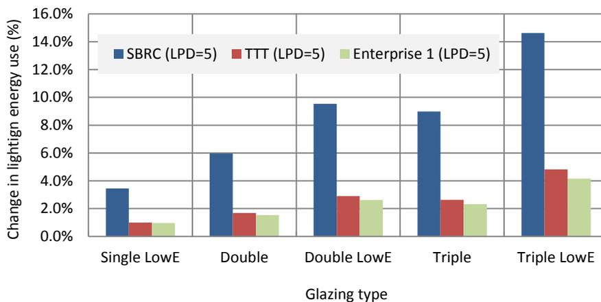
Figure 5-6 Glazing simulations: change in lighting energy use for identical LPD.
