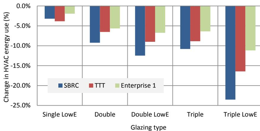
Figure 5-2 Glazing simulations: change in HVAC energy use.
