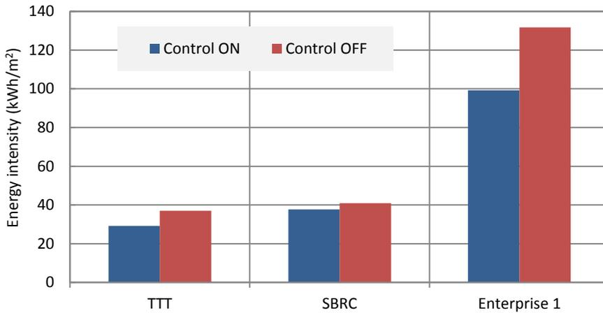
Figure 5-12 Lighting control simulations: yearly building energy use intensity.
