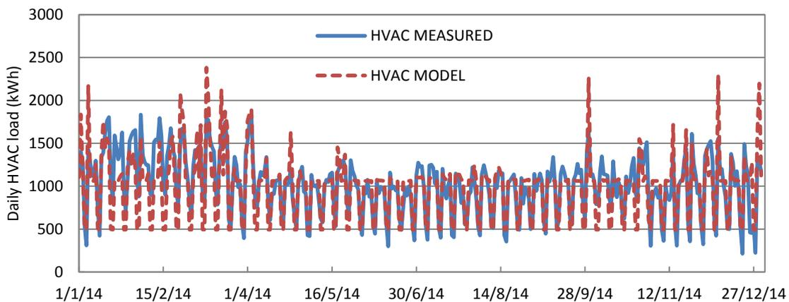
Figure 4-27 Enterprise 1 HVAC electrical use comparison.
