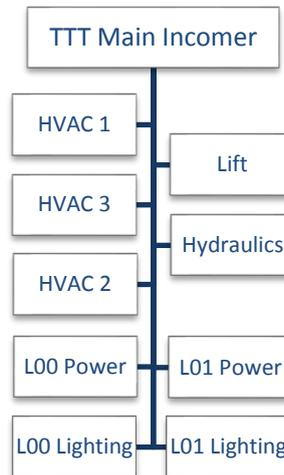
Figure 3-15 TTT electrical meters and sub-meters.
