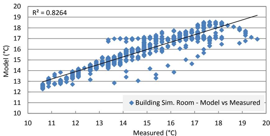
Figure 4-8  $R^2$  for building simulation room temperature comparison.
