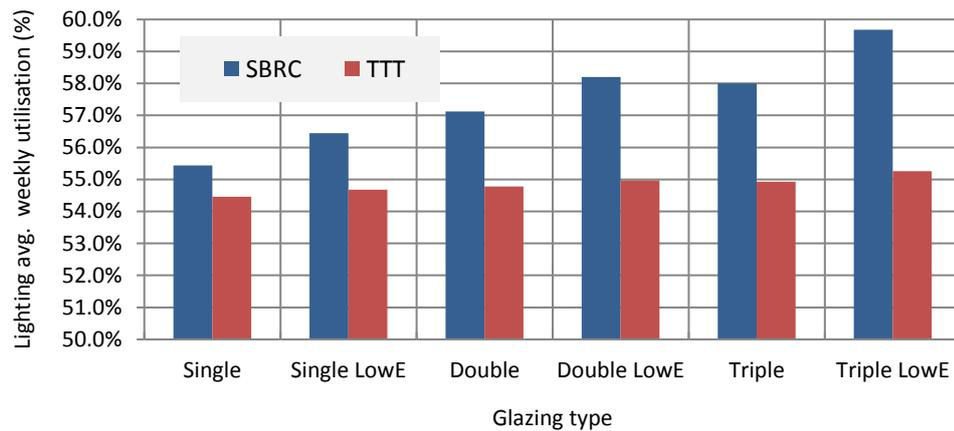
Figure 5-7 Glazing simulations: lighting system average weekly utilisation rates.
