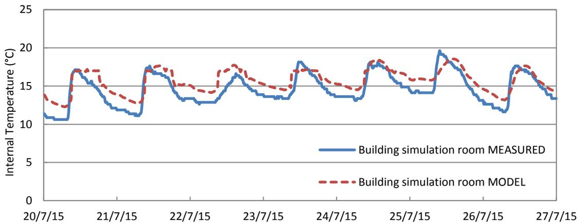
Figure 4-7 TTT Building simulation room temperature profile comparison.
