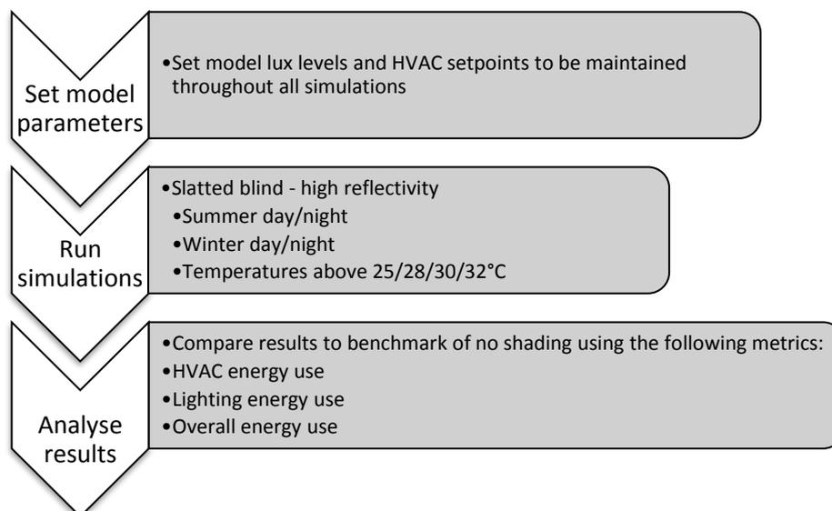
Figure 3-7 Window shading simulation procedure.
