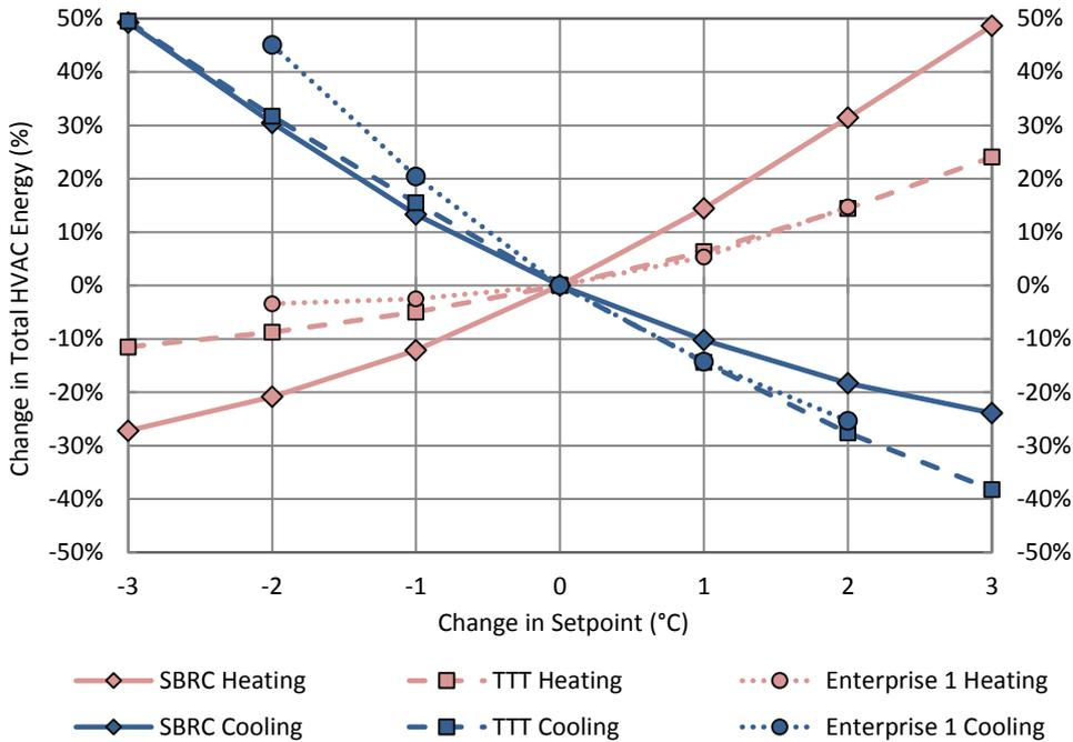
Figure 5-23 HVAC setpoint simulations: change in HVAC energy use.
