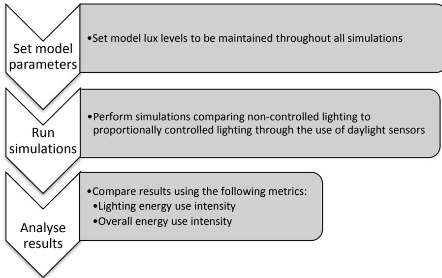
Figure 3-4 Lighting simulation procedure.
