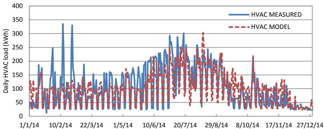
Figure 4-25 SBRC HVAC electrical use comparison.
