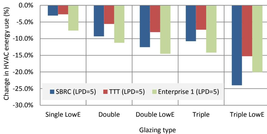
Figure 5-5 Glazing simulations: change in HVAC energy use for identical LPD.
