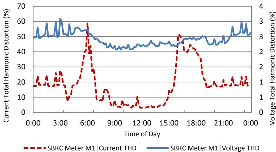
Figure 6-13 SBRC THD of voltage and current on a typical day.
