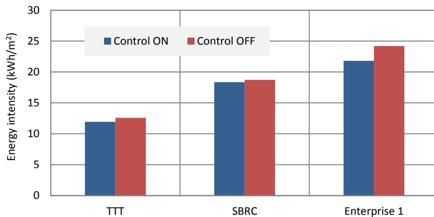
Figure 5-11 Lighting control simulations: yearly HVAC energy use intensity.
