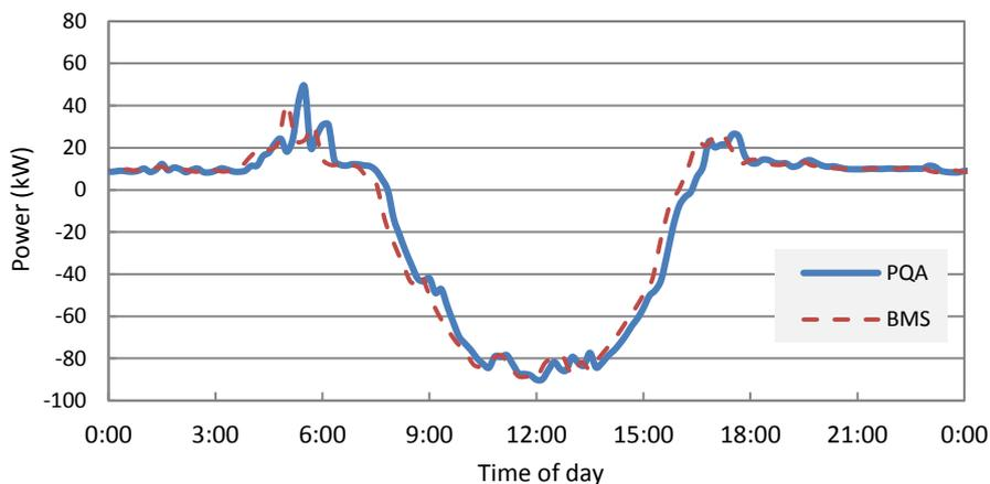
Figure 6-6 Power profile comparison as measured by BMS & PQA: 5/07/2015.
