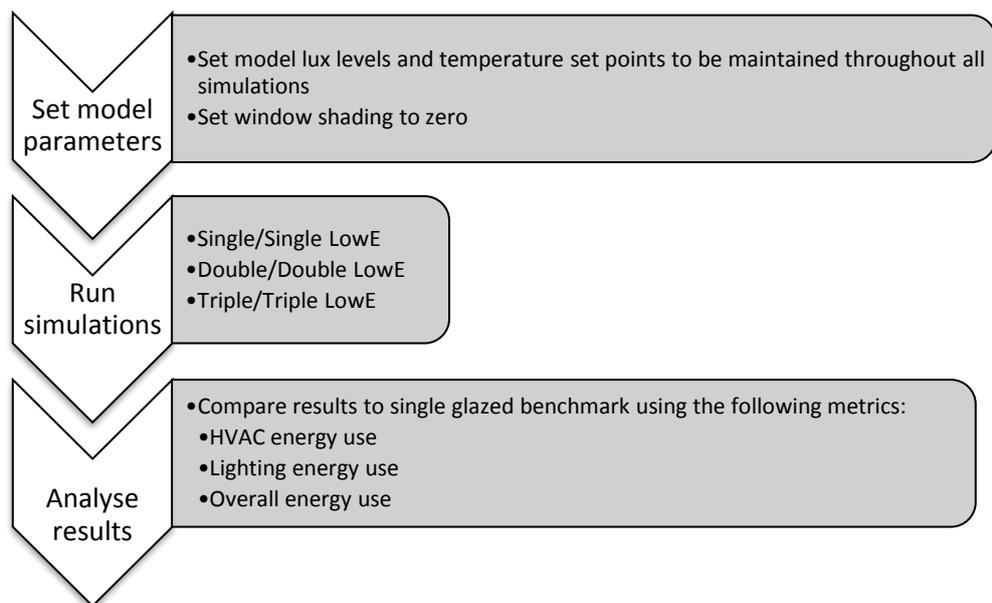
Figure 3-3 Glazing simulation procedure.
