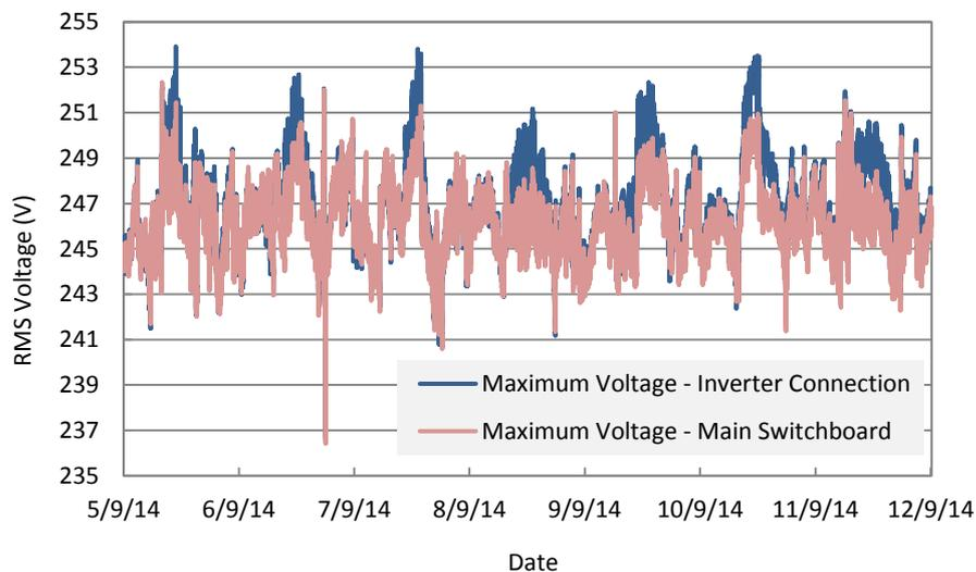
Figure 6-14 Maximum RMS voltage levels at the SBRC.
