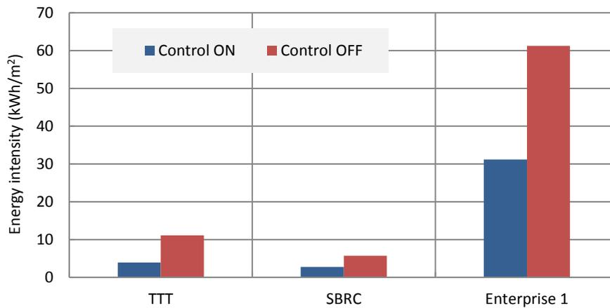
Figure 5-10 Lighting control simulations: yearly lighting energy use intensity.
