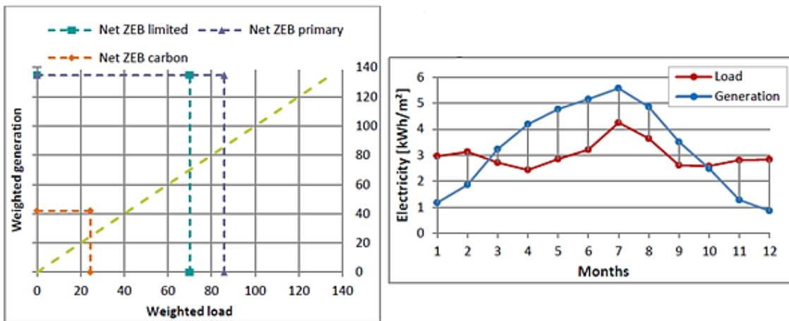
Figure B-3 NZEB balance for three definitions; Tracking of load/gen. - [17].
