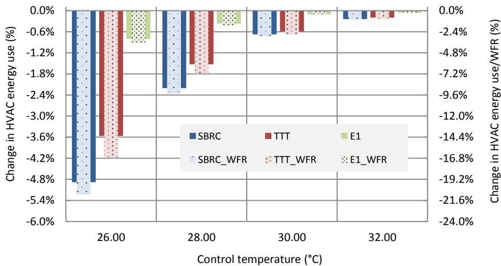
Figure 5-18 Shading simulations: HVAC energy use - temperature control.
