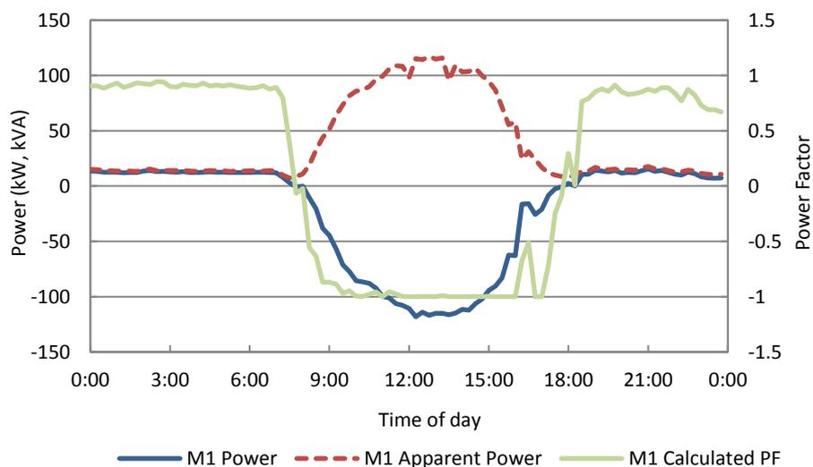
Figure 6-12 SBRC 15-minute average power factor, real, and apparent power.
