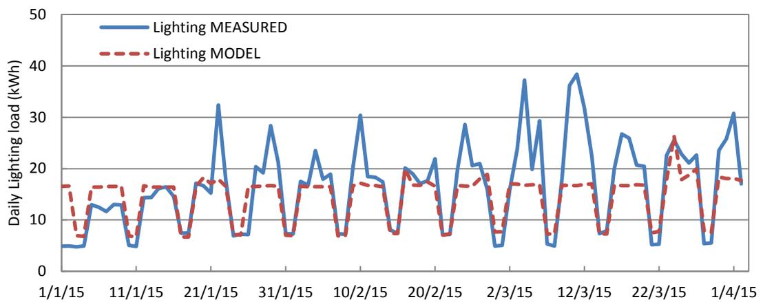
Figure 4-10 TTT lighting electrical use comparison.
