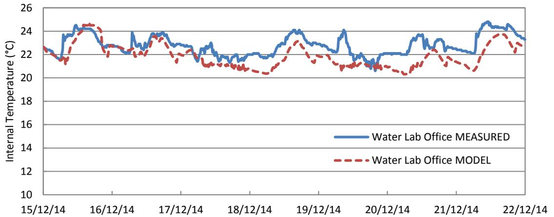
Figure 4-18 SBRC water lab office temperature profile comparison – summer.
