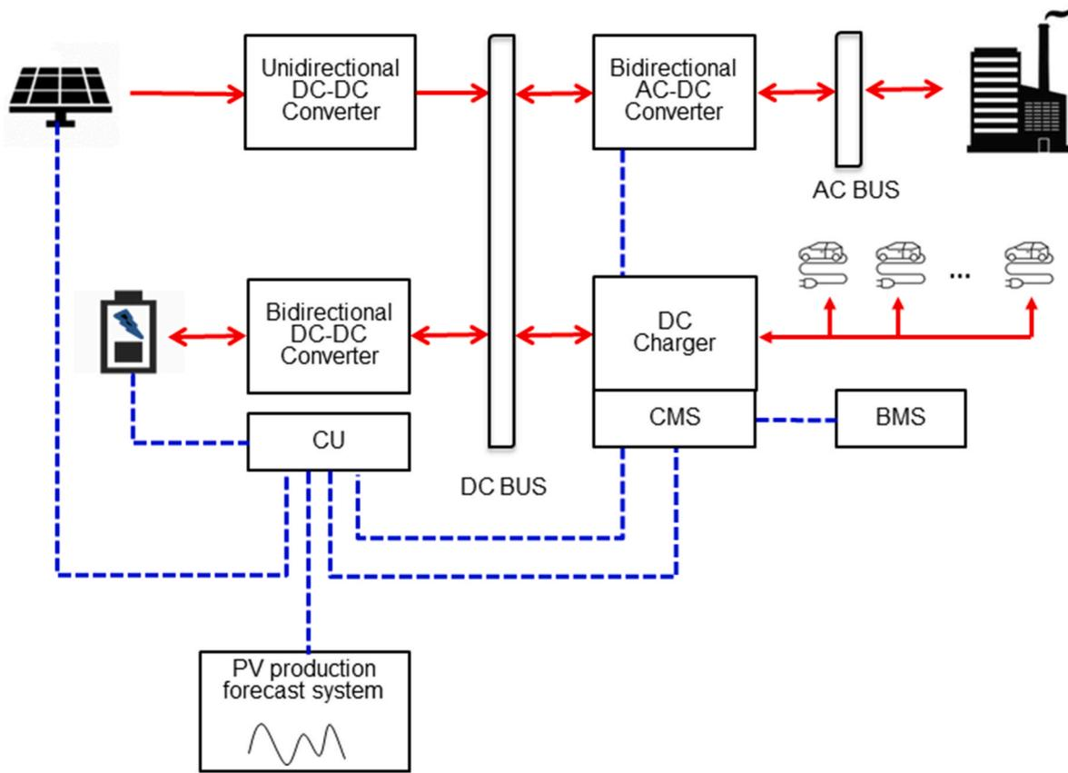
Fig. 1. Design of the emulated microgrid environment of a solar EV parking lot.
