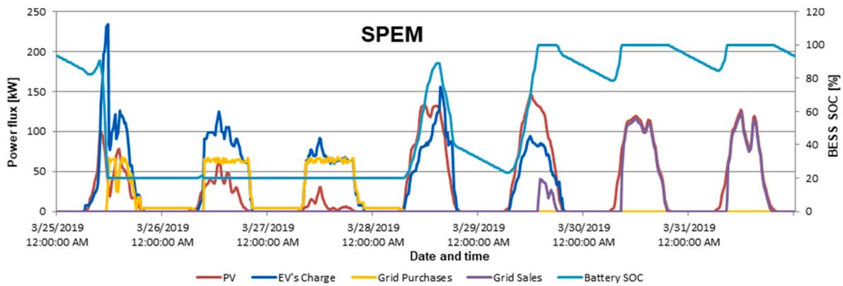
Fig. 8. One week time evolution (March 25–31, 2019) of the power fluxes profile output from SPEM design simulation. The different curves depict: the temporal evolution of power fluxes from PV (red), from grid purchase (yellow) and to grid sales (purple), the power provided for EV batteries charge (dark blue), BESS state of charge (light blue - on the right scale).
