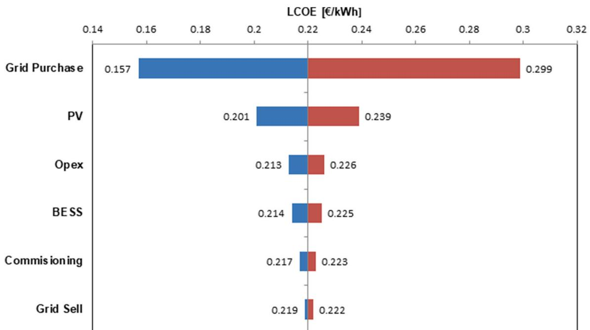
**Fig. 15.** Tornado diagram representing sensitivity analysis of ±50% variation from reference values to the final LCOE.
