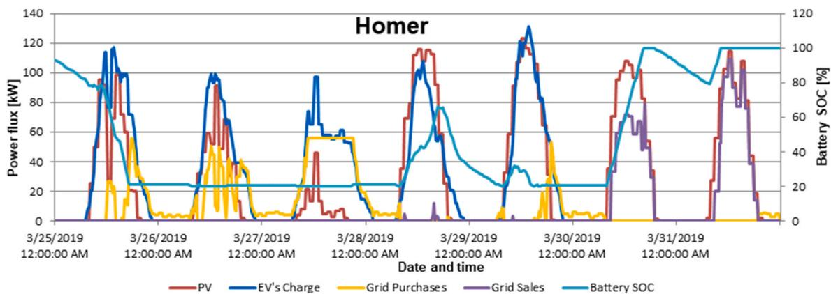
**Fig. 7.** One week time evolution (March 25–31, 2019) of the power fluxes profile output from HOMER® Grid simulation. The different curves depict: the temporal evolution of power fluxes from PV (red), from grid purchase (yellow) and to grid sales (purple), the power provided for EV batteries charge (dark blue), BESS state of charge (light blue - on the right scale).
