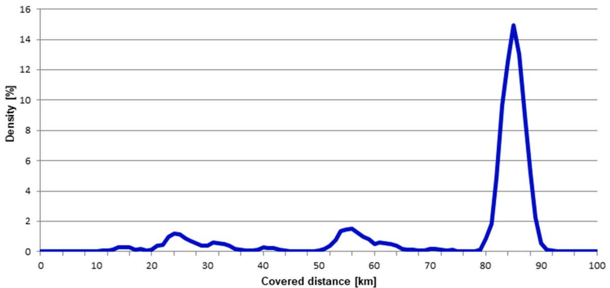
Fig. 6. Probability density function of EVs covered distance.
