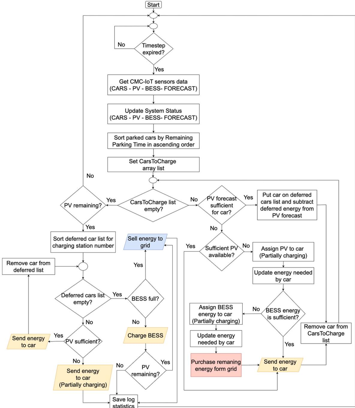
Fig. 3. Charging and deferring algorithm flowchart.
