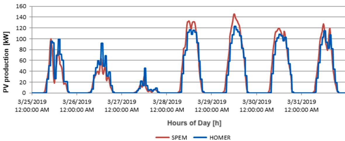
Fig. 9. The modeled PV output time evolution (March 25–31, 2019) in both simulations.
