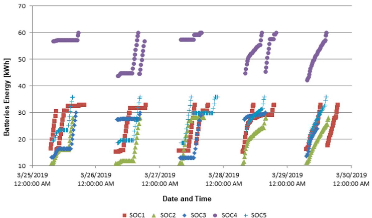
Fig. 14. SOC behavior of five different types of EVs with 28, 30, 33, 36 and 60 kWh battery associated with five different charging stations, obtained from SPEM simulation. Five working days (March 25–29, 2019) are represented; two different lines on the same days represent two EVs occupying the same slot.
