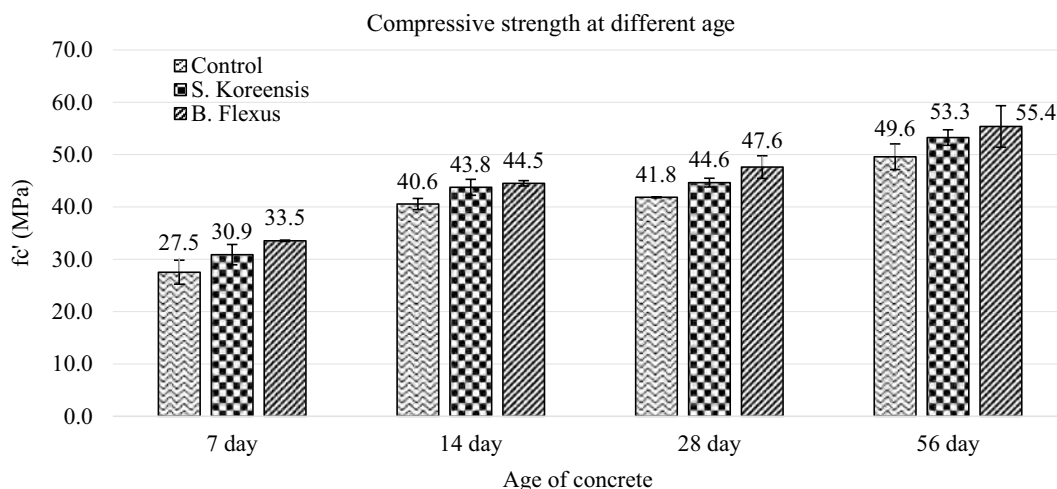
Fig. 2 Compressive strength of concrete at different age
