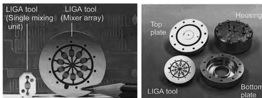
Fig. 24. Photographs of the mixer array: mixing parts made by an electroforming process in the frame of the LIGA process, single mixing unit and mixer array (top image); single and assembled pieces of the mixer array, mixer and housing consisting of top and bottom plates (bottom image).
