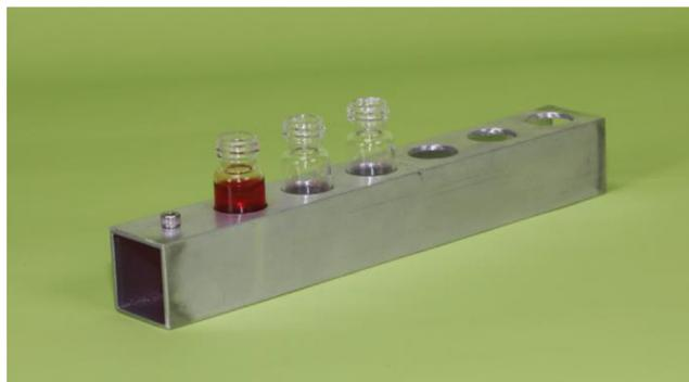
**Fig. 5.** An individual vial holder that can hold up to six 4 ml (1 dram) collection vials beneath each chromatography column. See the text and the **Design File** for details of dimensions and relative positions of the components used to build the rack.
