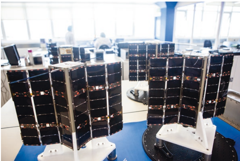
Fig. 5.5 A group of Spire’s Lemur satellites undergoing testing. (Image courtesy of Spire)
