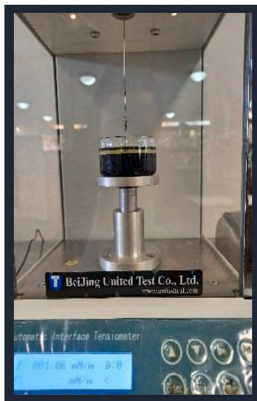
Fig. 2. Interfacial tension test. This picture shows the interphase between the flow enhancer and the crude oil at 25 °C.
