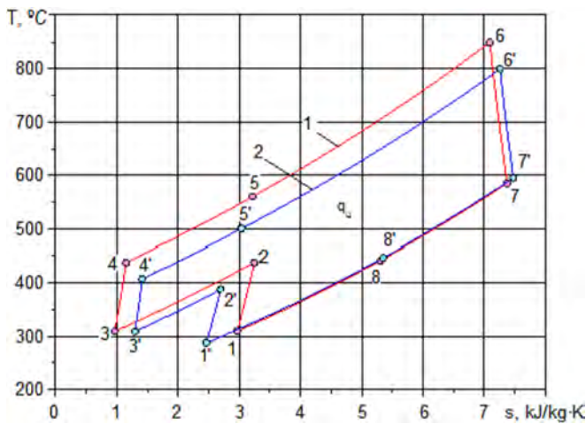
Fig. 6. T-s diagram of GT-MHR-250 plant. 1 – electricity generation mode, 2 – combined mode.
