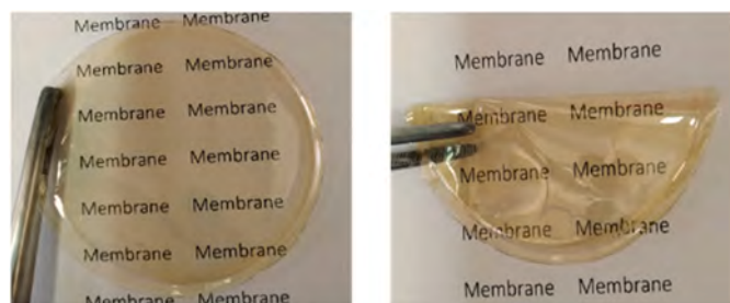
Fig. 3. Photographs of the prepared membranes based on P(IB-PEO)-20 copolymers indicating their transparency and flexibility.
