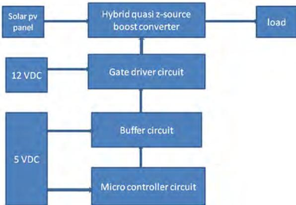
Fig. 3. Block diagram for Hybrid quasi-z-source boost converter.
