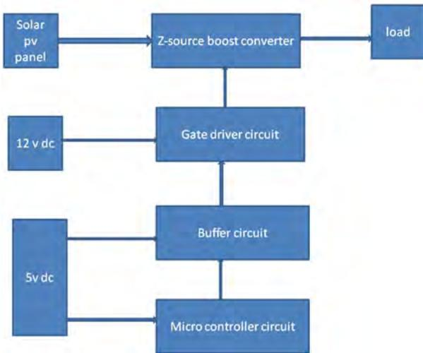
Fig. 2. Block diagram for z-source boost converter.
