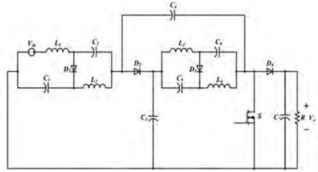
Fig. 4. Combination of two Quazi-Z-Source dc-dc Converter.
