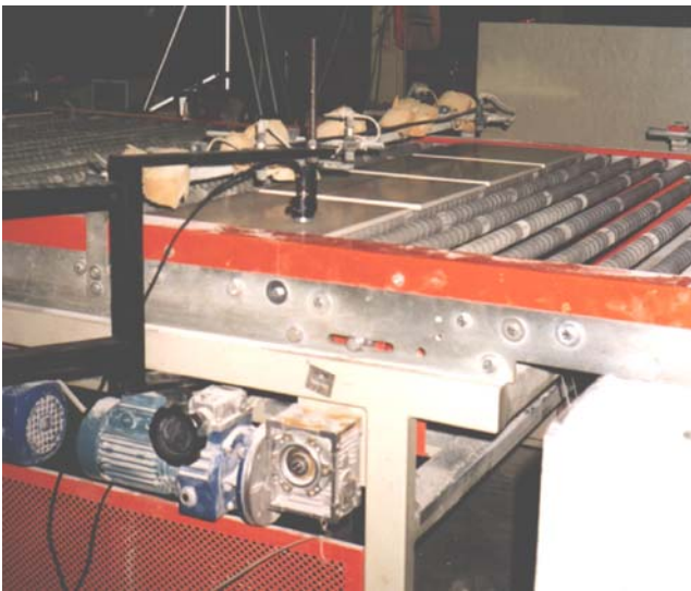
Fig. 6 Installation of the ultrasonic probes in the production line
