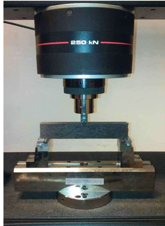
FIGURE 2: Three-point flexural strength test of a Formulation 1 sample.
