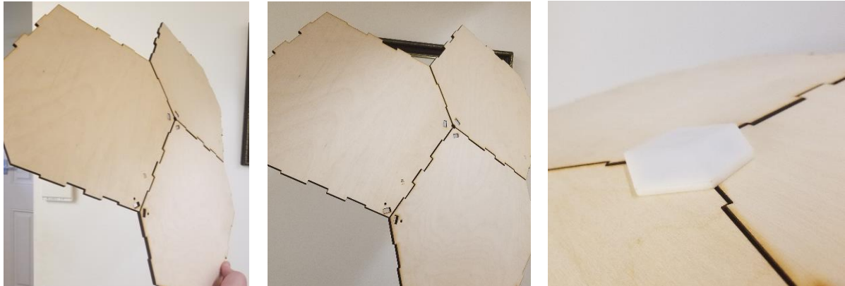
Figure 13: Fabricated panels in place with the first connection
