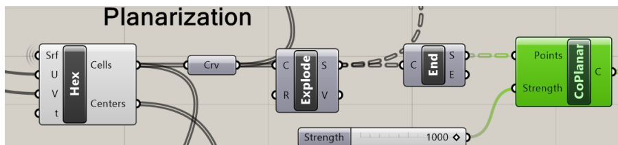
Figure 8: Planarization process and the CoPlanar component
