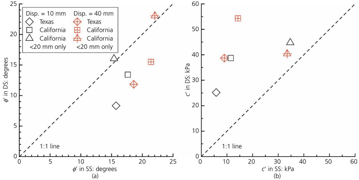
Figure 5. Comparison of shear strength parameters of MSW in SS and DS tests: (a) effective friction angle ( $\phi'$ ); (b) cohesion ( $c'$ ). Disp., displacement
