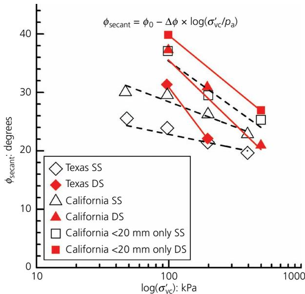
**Figure 7.** Relationship between vertical effective stress ( $\sigma'_{vc}$ ) in logarithmic scale and secant friction angle ( $\phi_{secant}$ ) at 40 mm displacement of waste specimens
