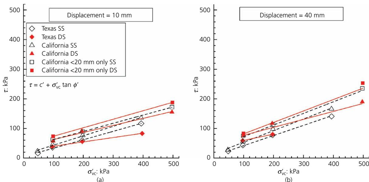
Figure 3. Relationships between vertical effective stress ( $\sigma'_{vc}$ ) and shear resistance ( $\tau$ ) of specimens at (a) 10 mm displacement and (b) 40 mm displacement
