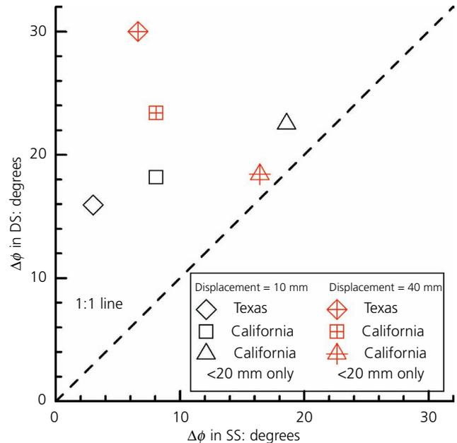
**Figure 8.** Comparison of change of secant friction angle of MSW with vertical effective stress ( $\Delta\phi$ ) in SS and DS tests
