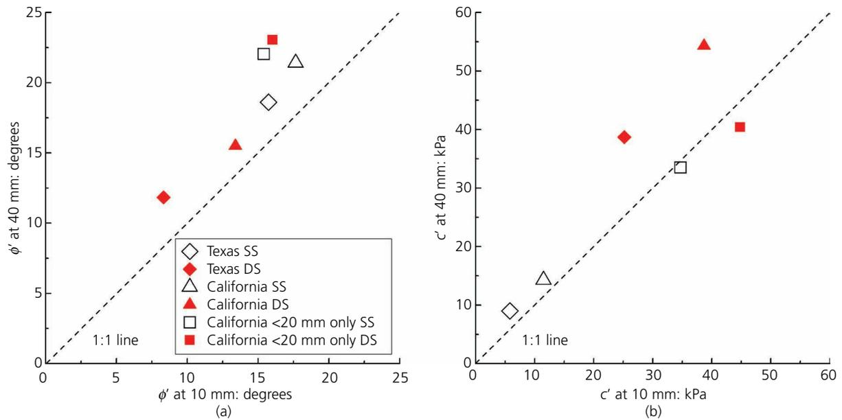
**Figure 4.** Comparison of shear strength parameters of MSW obtained at 10 and 40 mm displacements: (a) effective friction angle ( $\phi'$ ); (b) cohesion ( $c'$ )
