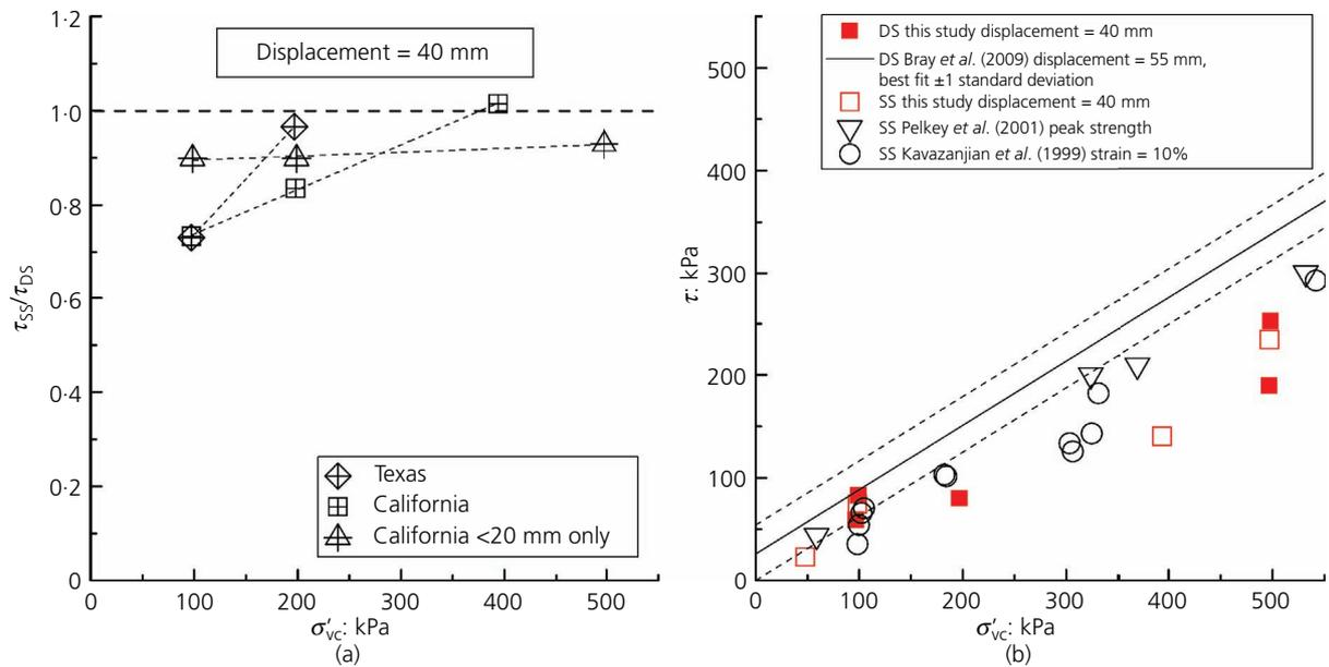
Figure 6. Relationships between vertical effective stress ( $\sigma'_{vc}$ ) and (a) ratio of shear strength between SS and DS tests ( $\tau_{SS}/\tau_{DS}$ ) at 40 mm displacement and (b) shear strength ( $\tau$ ) obtained from SS and DS tests in this study and in the literature based on different failure criteria
