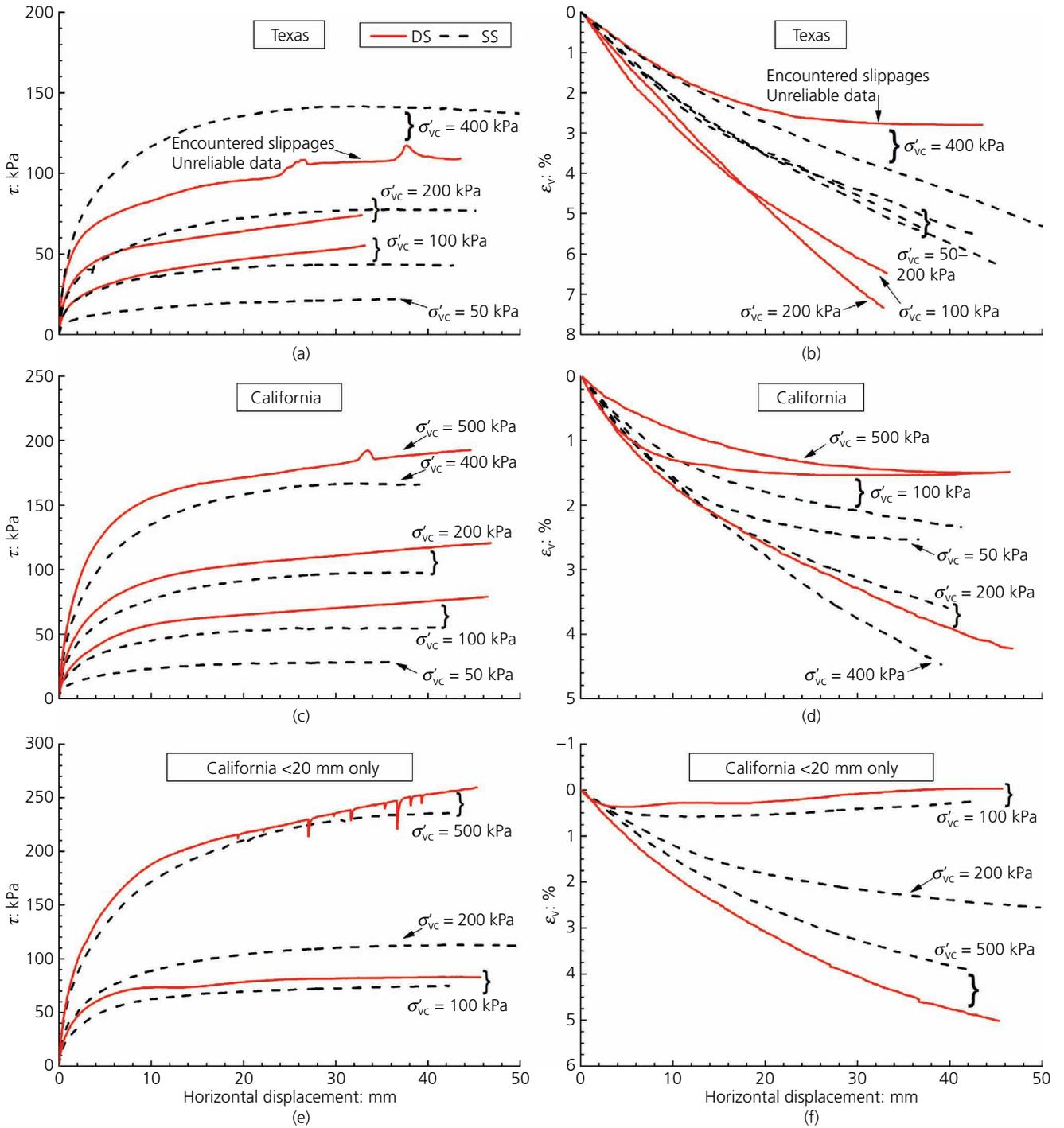
**Figure 2.** Shear responses of MSW specimens with horizontal displacement in DS (continuous lines) and SS (dashed lines) tests: (a) shear stress and (b) vertical strain of Texas waste; (c) shear stress and (d) vertical strain of California waste; and (e) shear stress and (f) vertical strain of California <20 mm only waste
