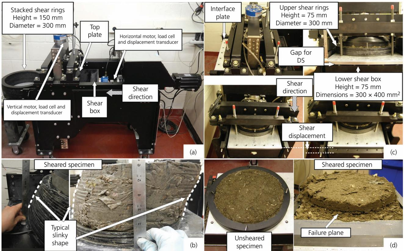
**Figure 1.** Schematic diagrams of test set-ups for DS and SS tests: (a) device for SS tests; (b) a sheared SS specimen; (c) device for DS tests; (d) unsheared and sheared DS specimens. LVDT, linear variable differential transformer
