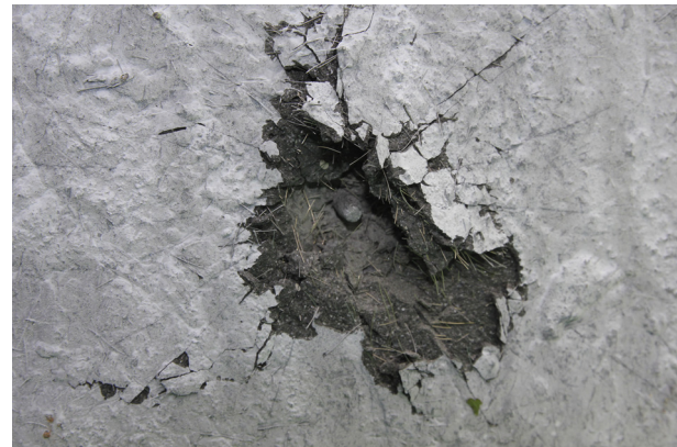
Fig. 4. Perforation limit: tip of the non-deformable projectile protrudes from the back side of the 50 mm thin UHPFRC 3-2 slab.
