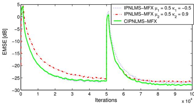
Figure 9: EMSE performance for the adaptive combination of two IPNLMS algorithms in a modified filtered-x ANC configuration (CIPNLMS-MFX). Component settings are shown in the legend.
