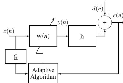
Figure 2: Conventional filtered-x (FX) structure for ANC.
