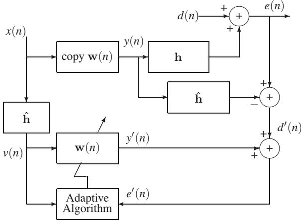
Figure 3: Modified filtered-x (MFX) structure for ANC.
