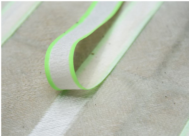
Figure 16: Resin on fiberglass masked off using tape
