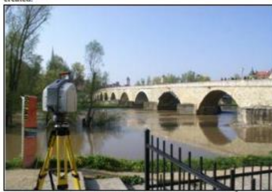
Time of Flight system used for capturing long distance object 7
