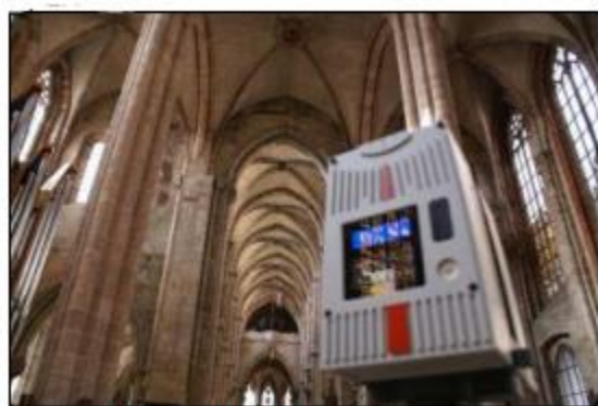
Phase based System used at interior scanning 8
