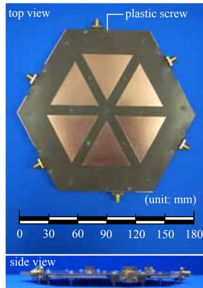
Fig. 4 Fabricated antenna
