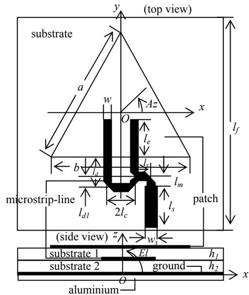
Fig. 2 Configuration of single triangular patch antenna
