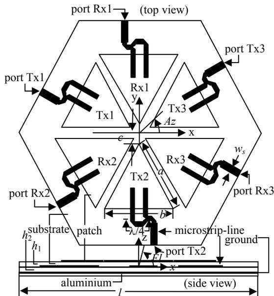
Fig. 3 A dual band equilateral triangular-patch array antenna
