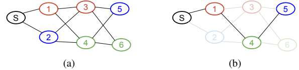
Fig. 1: (a) A deployment with multiple correlated sensor groups (denoted by colors), and (b) coverage of the entire monitoring region by a subset of connected active nodes.
