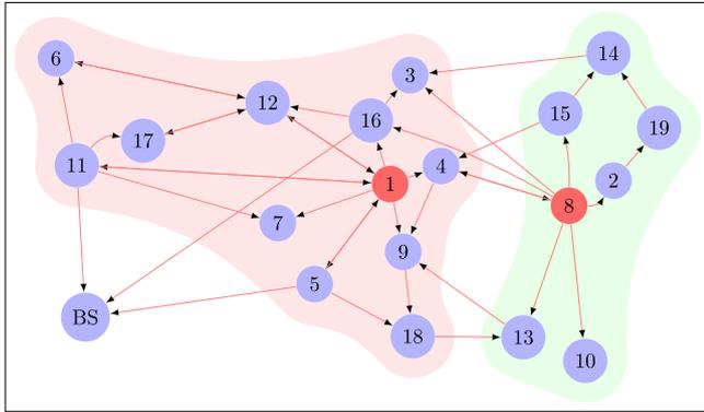
Fig. 1. A random 20 sensor node network with 2 cluster heads (1 and 8).
