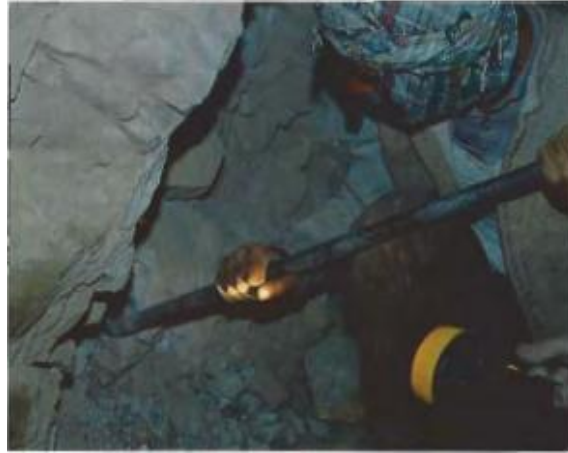
Figure 9. Picks and crowbars are also used in the mine to remove loosened wallrock. Photo by Gary Bowersox.
