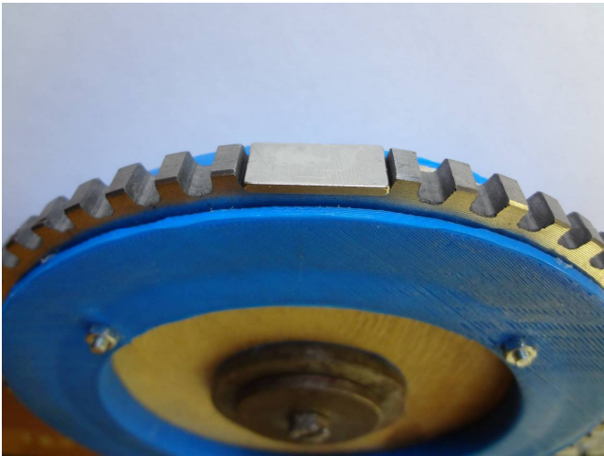
Fig. 12. The magnet position on the pulley.
