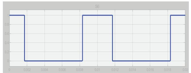
Fig. 27. Switching pattern for switch S6
