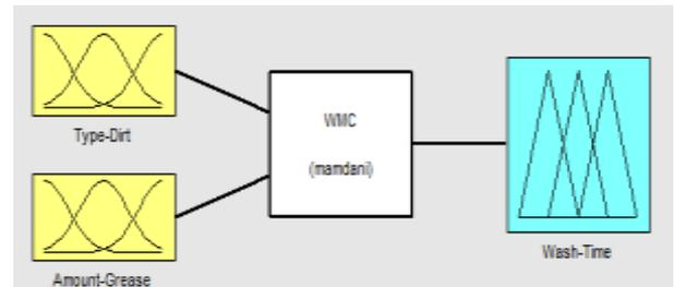
Fig 3: FLC for an automatic domestic washing machine
