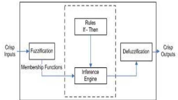
Fig 1: Basic block diagram of a Fuzzy Logic Controller (FLC)
