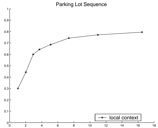
Figure 10: Parking Lot Sequence: The ROC curve shows the performance of the local context detector. The object-centered approach fails because faces are too small in this sequence, so its ROC is not shown. The local context detector retrieves about 75% of the actual faces at 7 false alarms per frame. This clearly indicates that the local context detector goes beyond the capabilities of object-centered face detectors.
