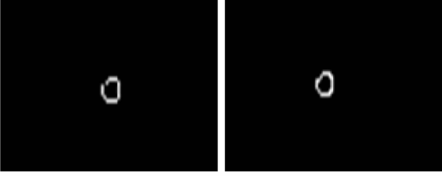
Fig. 9. (a) Defects before dilation and erosion (b) Image after removing discontinuity of bright pixels using dilation and erosion.
