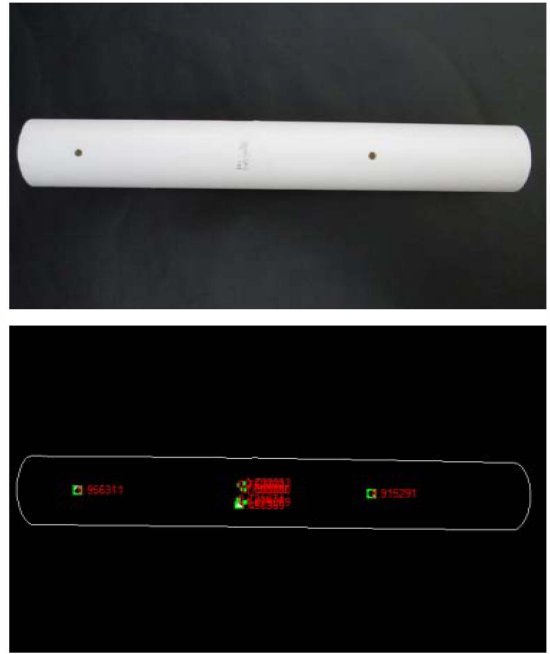
Fig. 14. Input RGB image. In this image there are two holes and one big crack. (b) Output of proposed algorithm. The holes are identified accurately but the crack is not identified correctly due to the presence of discontinuity.
