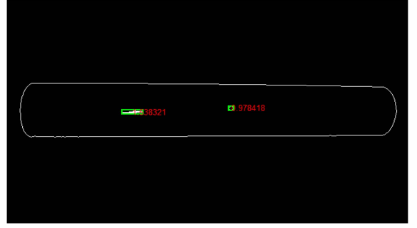
Fig. 11. Output of proposed algorithm. One small crack and a small hole are identified accurately according to their area to perimeter ratio. These are represented by a minimum bounding rectangle that tightly bounds the defects.
