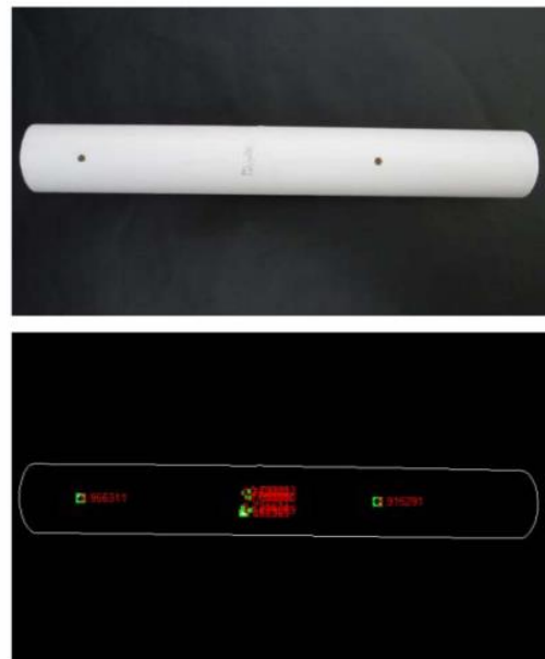
Fig. 14. Input RGB image. In this image there are two holes and one big crack. (b) Output of proposed algorithm. The holes are identified accurately but the crack is not identified correctly due to the presence of discontinuity.
