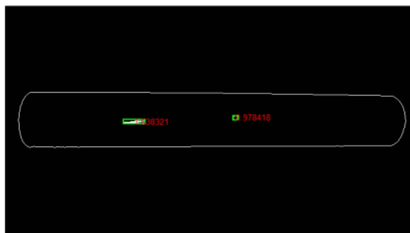
Fig. 11. Output of proposed algorithm. One small crack and a small hole are identified accurately according to their area to perimeter ratio. These are represented by a minimum bounding rectangle that tightly bounds the defects.
