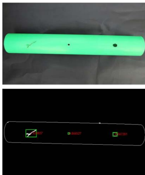
Fig. 12. (a) Input RGB image. In this image there are three defects include two hole and one crack. (b) Output of the proposed algorithm. All the defects are identified correctly according to their area to perimeter ratio and tightly bounded by minimum rectangle.
