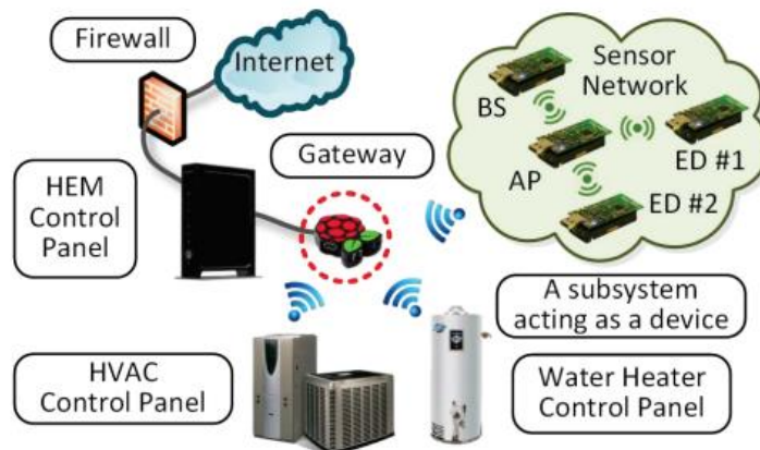
Fig. 2. The Hardware Architecture of the Fog Computing Platform for HEM.
