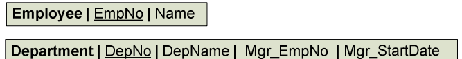
Fig 3. Extra algorithm adjustments made to the transformed RDS in Fig 1. The attributes “EmpNo” and “StartDate” have been re-named to Mgr_EmpNo and “Mgr_StartDate”. The abbreviated prefix “Mgr” represents the word “Manager”
